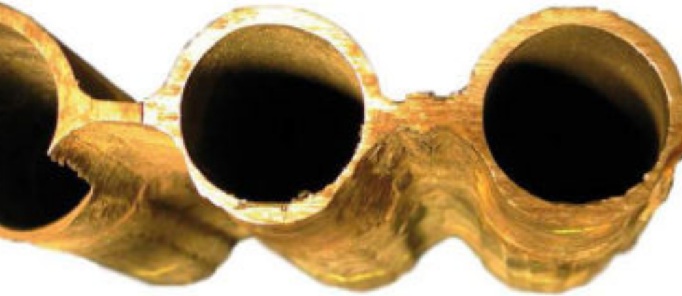
Finned boiler tubes
